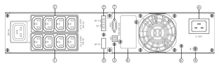
Figure 11: Rear view of PowerValue 11 RT 3 kVA B
