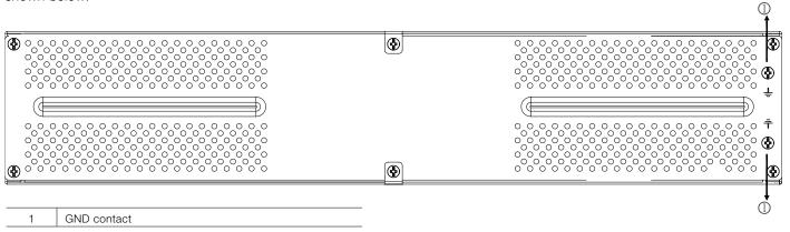
Figure 13: Rear view of 36V, 48V and 72V Battery Enclosures
