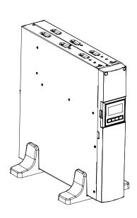
Figure 5: Installing the UPS in a vertical position
