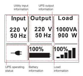
Figure 16: The default LCD display
