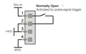
Figure 25: Input Dry contact schematic
