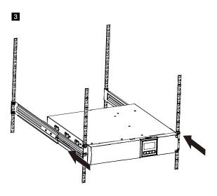
Figure 2: Installing the UPS
