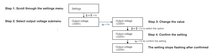
Figure 23: Setting rated output voltage value
