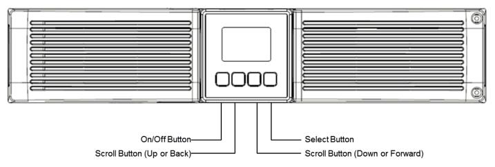
Figure 8: UPS front panel
