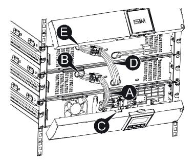
Figure 4: Installing multiple external battery enclosures
