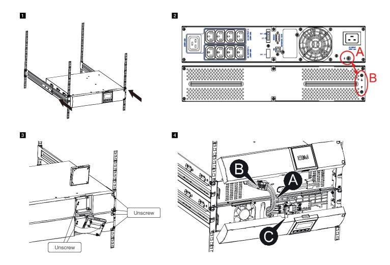
Figure 3: Installing the external battery enclosure
