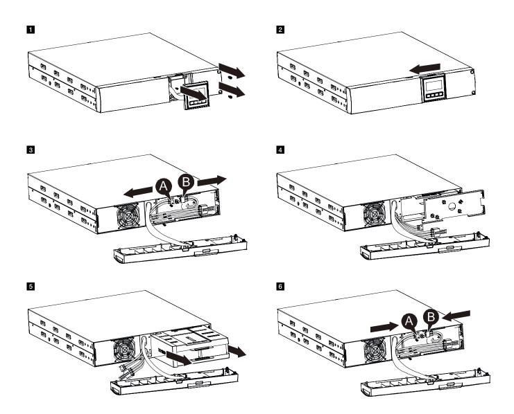
Figure 1: Replacing internal batteries
